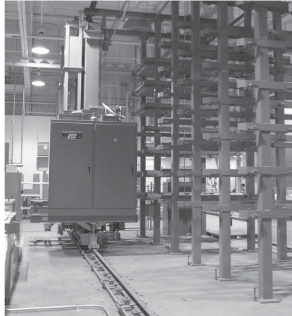
This ASRS stores many different types of metal that is stored and retrieved as required for a router operation. Material and router operations are all fully computerized.
