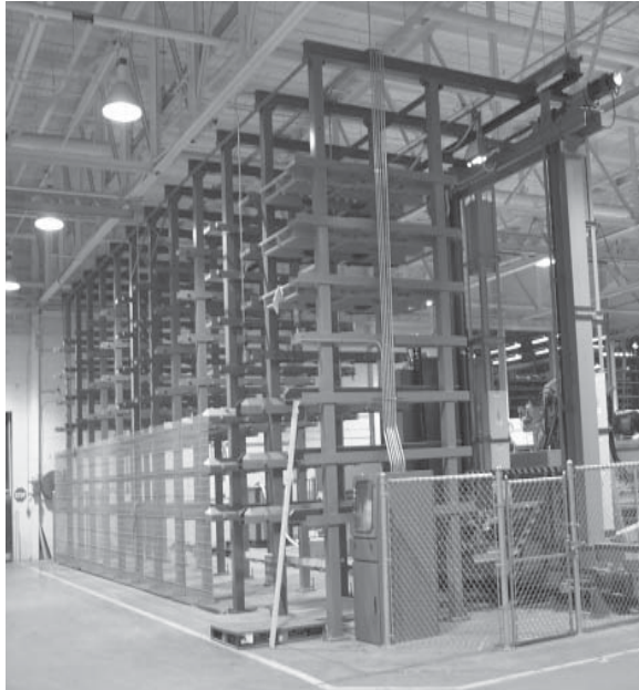
This ASRS stores many different types of metal that is stored and retrieved as required for a router operation. Material and router operations are all fully computerized.
